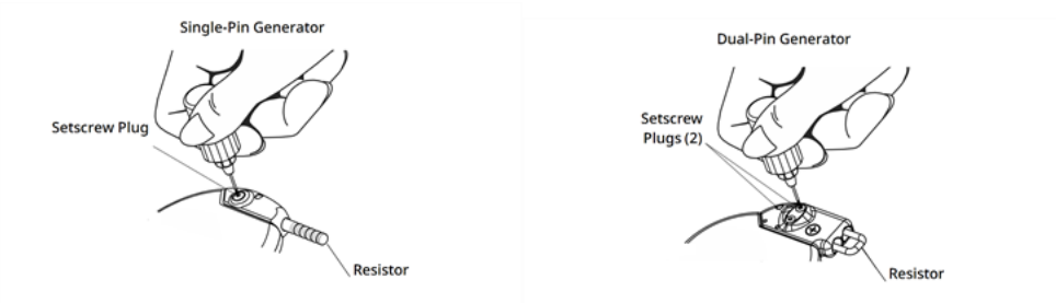
Figure 42. Resistor Assembly Connection for Single and Dual Receptacle Generators
