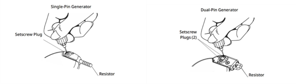
Figure 38. Connect the Resistor Assembly
